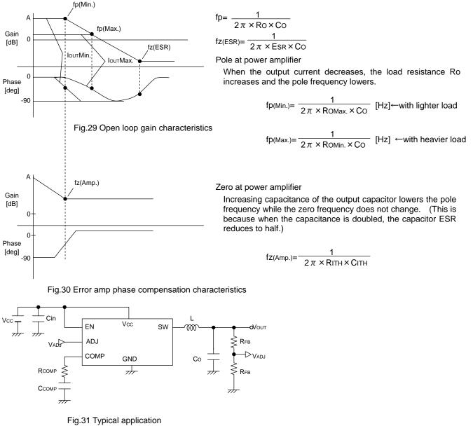
Stable feedback loop may be achieved by canceling the pole fp (Min.) produced by the output capacitor and the load resistance with CR zero correction by the error amplifier.
