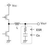
Fig.27 Output capacitor
