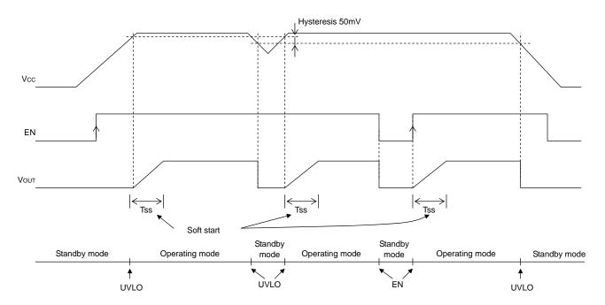
Fig.20 Soft start, Shutdown, UVLO timing chart
