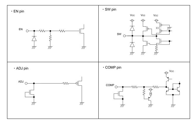
Fig.36 I/O equivalence circuit
