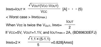
A low ESR 22µF/10V ceramic capacitor is recommended to reduce ESR dissipation of input capacitor for better efficiency.
