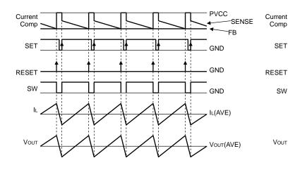
Fig.19 PWM switching timing chart
