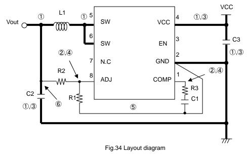
(1)To avoid conduction loss, please keep Black thick line as short and thick as possible.
