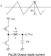
The inductance significantly depends on output ripple current. As seen in the equation (1), the ripple current decreases as the inductor and/or switching frequency increases.
