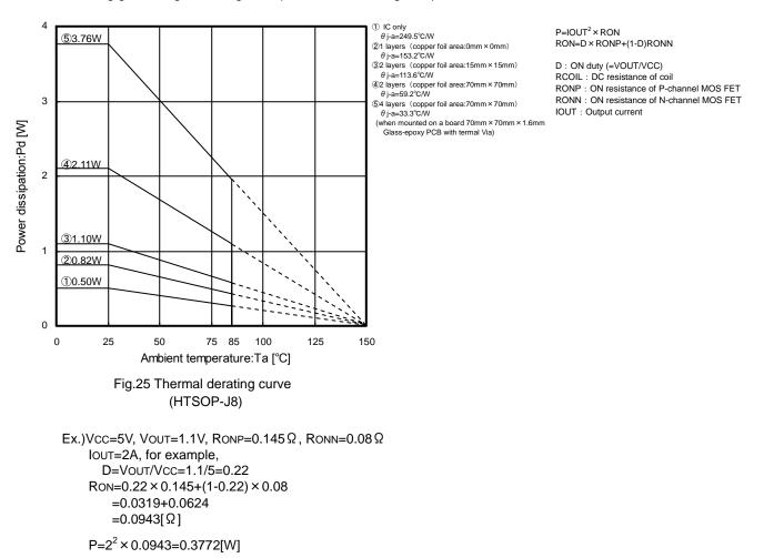
As RONP is greater than RONN in this IC, the dissipation increases as the ON duty becomes greater. With the consideration on the dissipation as above, thermal design must be carried out with sufficient margin allowed.
