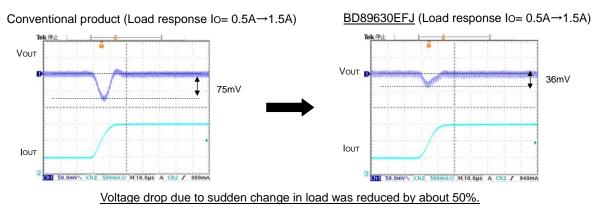
Fig.22 Comparison of transient response
