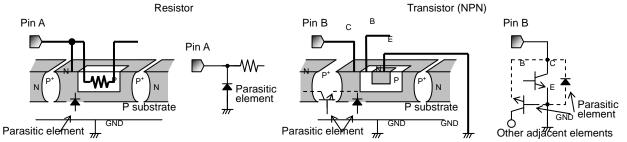
Fig.37 Simplified structure of monorisic IC
