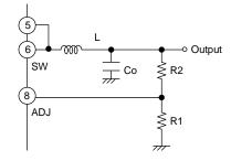
Fig.32 Determination of output voltage
