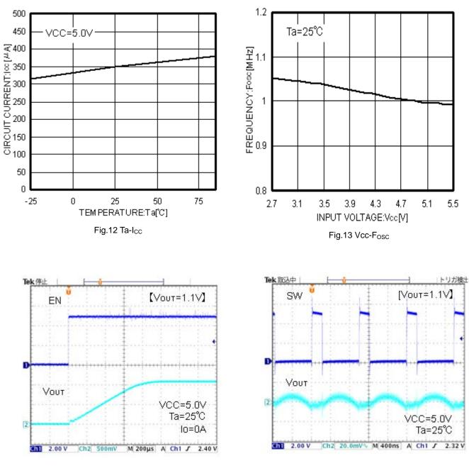
Fig.14 Soft start waveform
