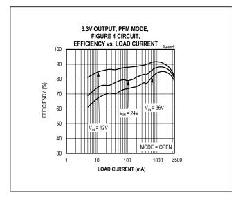
Figure 4. MAX17544 3.3V Output Efficiency (PFM Mode)
