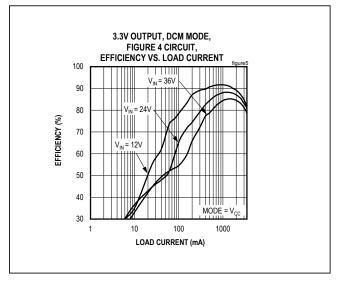
Figure 5. MAX17544 3.3V Output Efficiency (DCM Mode)
