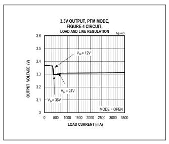
Figure 3. MAX17544 3.3V Output Load and Line Regulation (PFM Mode)
