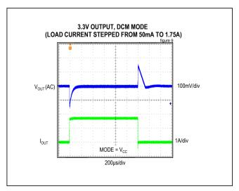
Figure 9. MAX17544 3.3V Output, 50mA to 1.75A Load Transient (DCM Mode)
