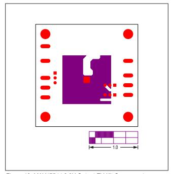
Figure 18. MAX17544 3.3V Output EV Kit Component Placement Guide—Bottom Solder Mask
