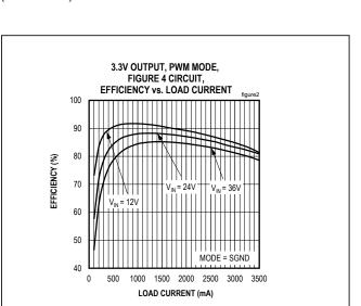
Figure 2. MAX17544 3.3V Output Efficiency (PWM Mode)
