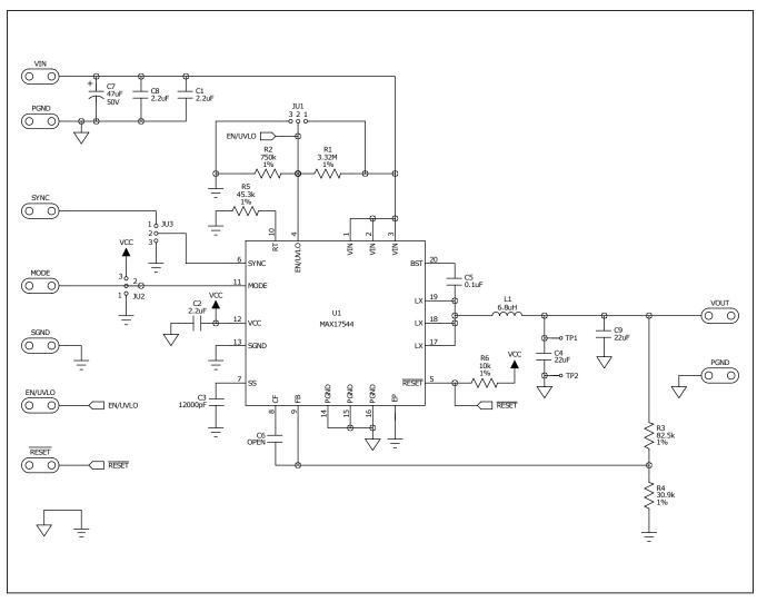
Figure 11. MAX17544 3.3V Output EV Kit Schematic
