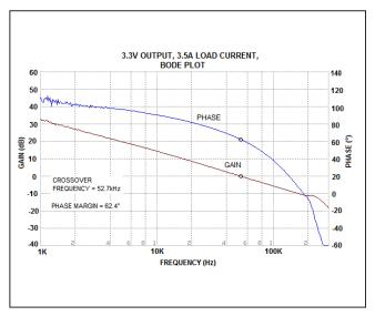
Figure 6. MAX17544 3.3V Output Full Load Bode Plot ( $V_{IN} = 24V$ )
