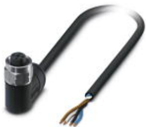
Sensor/Actuator cable, 4-position, PE-X halogen-free, black-gray RAL 7021, free cable end, on Socket angled M12, A-coded, Cable length: 10 m, for outdoor applications, with high-grade steel knurl
